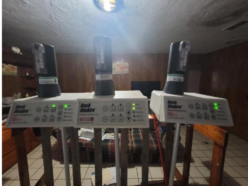
Calibration prior to testing
